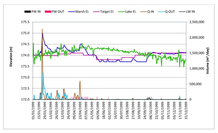
Figure 2: Daily Water Levels, flows and Pumping Water Plot for Open Water Marsh in a Dry Year, 1999 Condition
