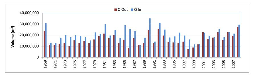
Figure 42: Streamflow Entered into and Water Released from the Marsh under Open Water 2 Marsh Scenario
