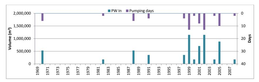
Figure 47: Water Quantity Pumped into the Marsh and Pumping Days under Hemi Marsh Scenario
