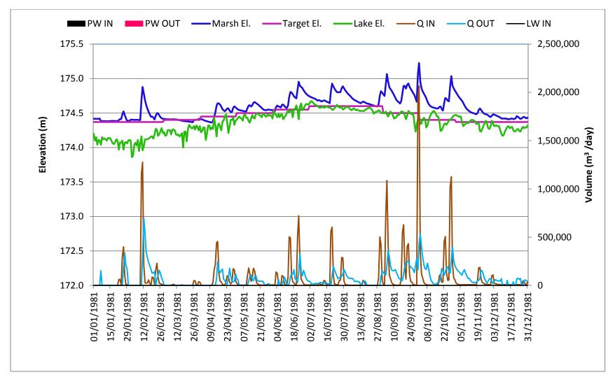
Figure 35: Daily Water Levels, flows and Pumping Water Plot for Overgrown Marsh in a Wet Year, 1981 Condition
