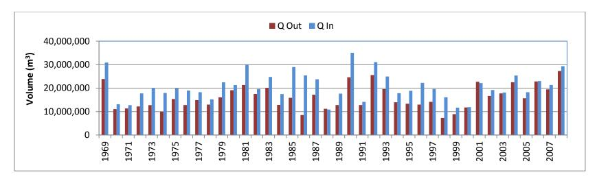
Figure 43: Streamflow Entered into and Water Released from the Marsh under Hemi Marsh Scenario
