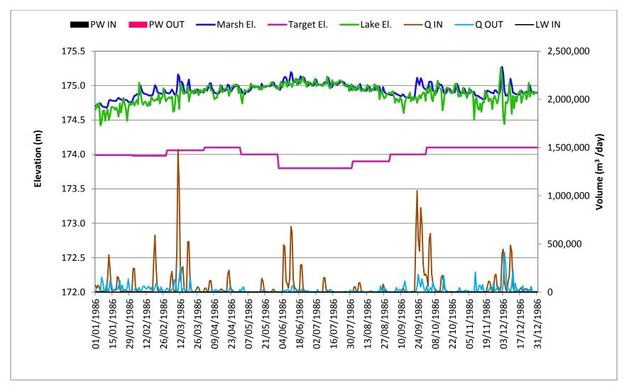
Figure 7: Daily Water Levels, flows and Pumping Water Plot for Open Water Marsh in a Wet Year, 1986 Condition
