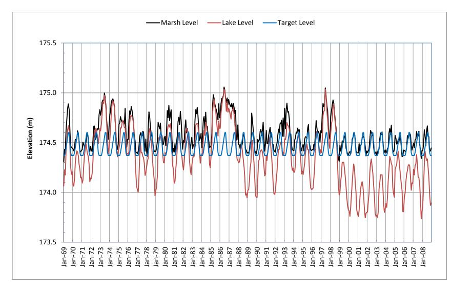
Figure 40: Monthly Average Marsh and Lake Levels during 1969 to 2008 and Target Levels for Overgrown Marsh Phase
