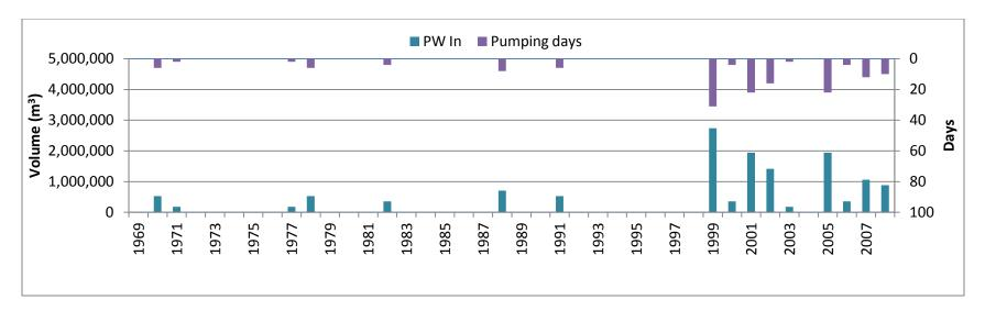
Figure 45: Water Quantity Pumped into the Marsh and Pumping Days under Open Water Marsh Scenario
