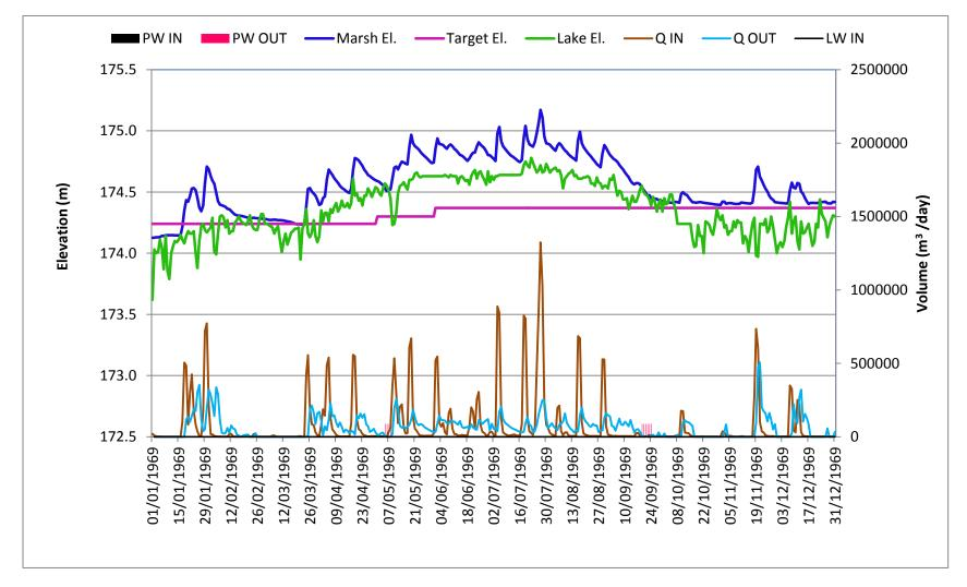
Figure 27: Daily Water Levels, flows and Pumping Water Plot for Hemi Marsh in a Wet Year, 1981 Condition
