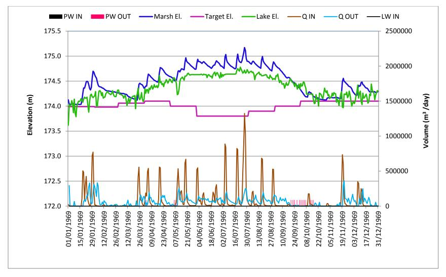
Figure 9: Daily Water Levels, flows and Pumping Water Plot for Open Water Marsh in a Wet Year, 1969 Condition
