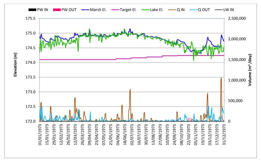
Figure 15: Daily Water Levels, flows and Pumping Water Plot for Open Water 2 Marsh in an Average Year, 1973 Condition
