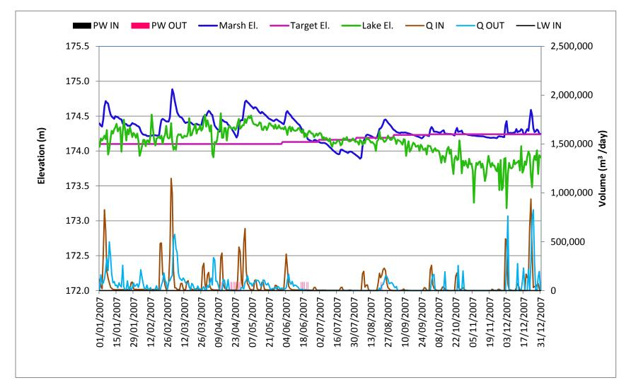
Figure 13: Daily Water Levels, flows and Pumping Water Plot for Open Water 2 Marsh in an Average Year, 2007 Condition
