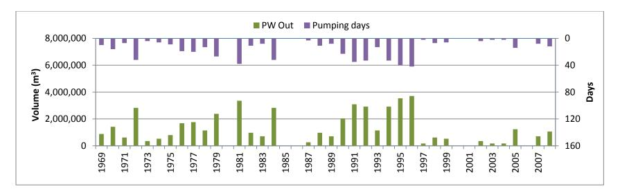
Figure 49: Water Quantity Pumped out from the Marsh and Pumping Days under Open Water Marsh Scenario
