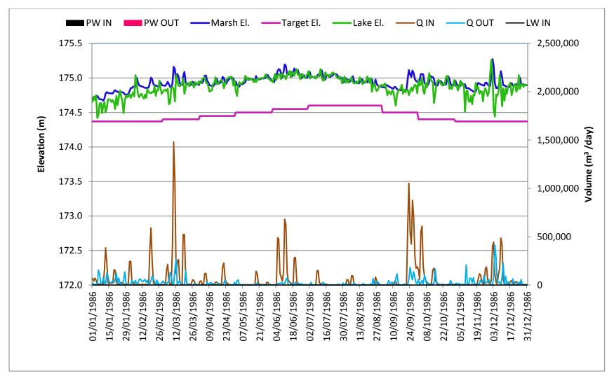
Figure 34: Daily Water Levels, flows and Pumping Water Plot for Overgrown Marsh in a Wet Year, 1986 Condition
