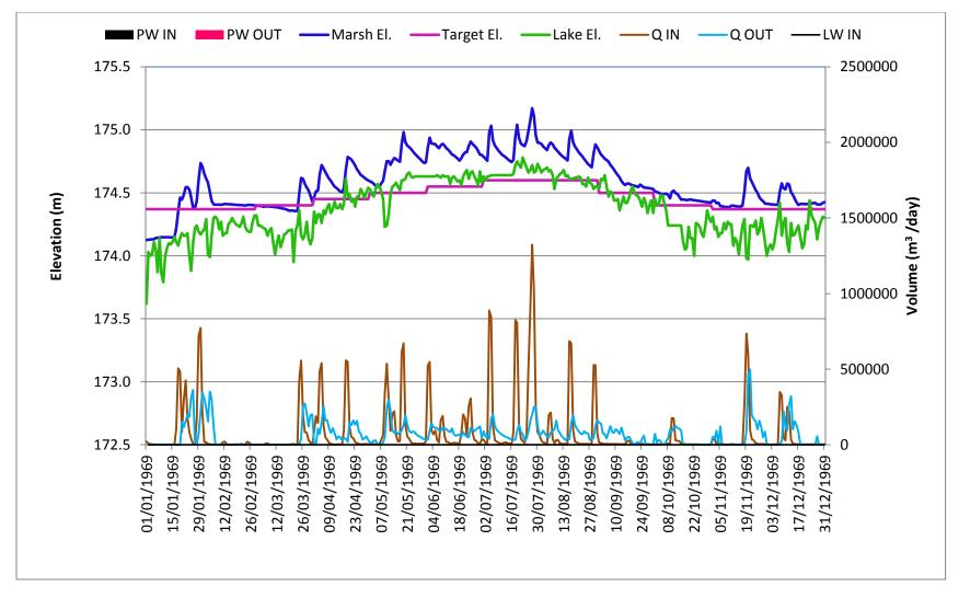
Figure 36: Daily Water Levels, flows and Pumping Water Plot for Overgrown Marsh in a Wet Year, 1969 Condition
