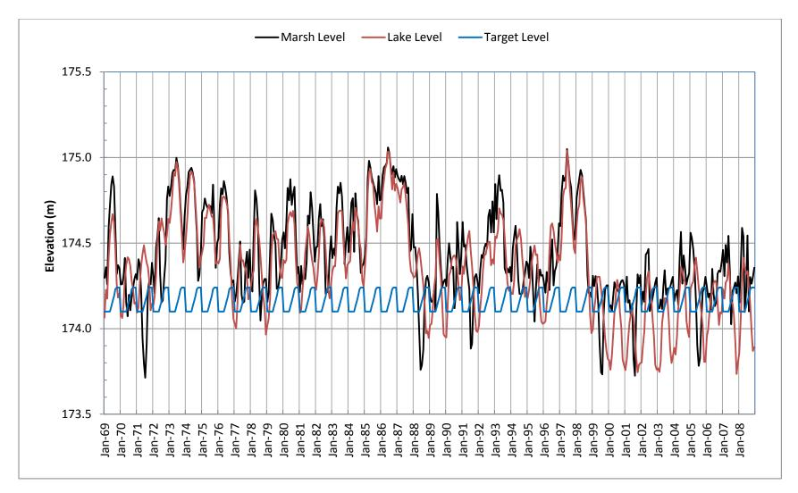
Figure 38: Monthly Average Marsh and Lake Levels during 1969 to 2008 and Target Levels for Open Water 2 Marsh Phase
