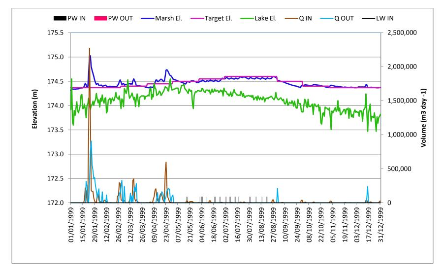
Figure 29: Daily Water Levels, flows and Pumping Water Plot for Overgrown Marsh in a Dry Year, 1999 Condition
