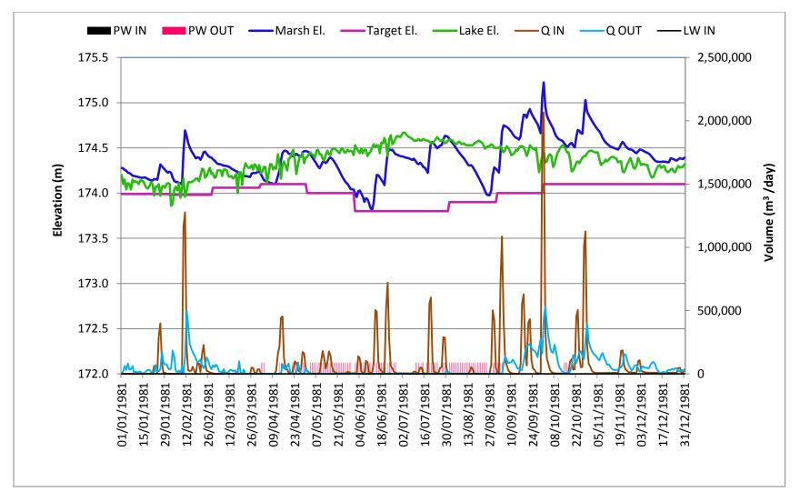
Figure 8: Daily Water Levels, flows and Pumping Water Plot for Open Water Marsh in a Wet Year, 1981 Condition
