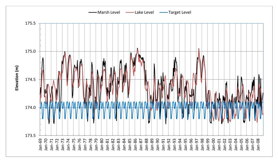
Figure 37: Monthly Average Marsh and Lake Levels during 1969 to 2008 and Target Levels for Open Water Marsh Phase
