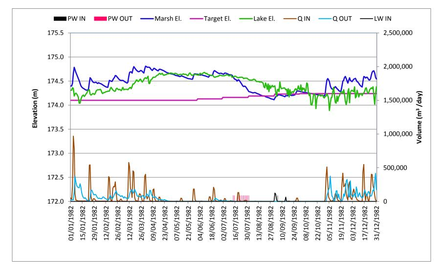
Figure 12: Daily Water Levels, flows and Pumping Water Plot for Open Water 2 Marsh in a Dry Year, 1982 Condition
