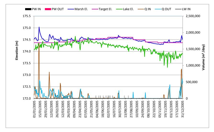
Figure 28: Daily Water Levels, flows and Pumping Water Plot for Overgrown Marsh in a Dry Year, 2005 Condition
