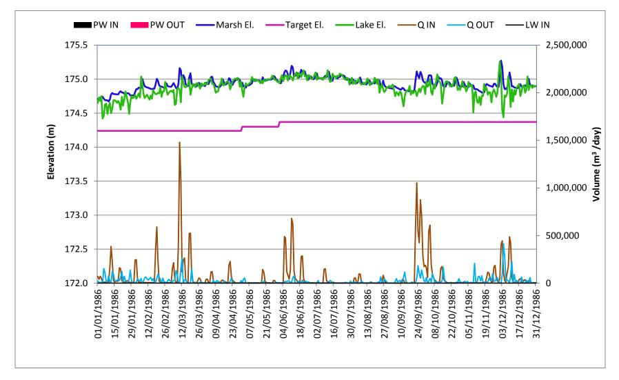
Figure 25: Daily Water Levels, flows and Pumping Water Plot for Hemi Marsh in a Wet Year, 1986 Condition
