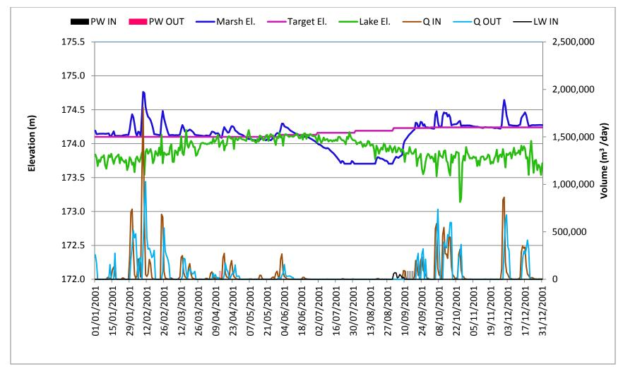
Figure 14: Daily Water Levels, flows and Pumping Water Plot for Open Water 2 Marsh in an Average Year, 2001 Condition
