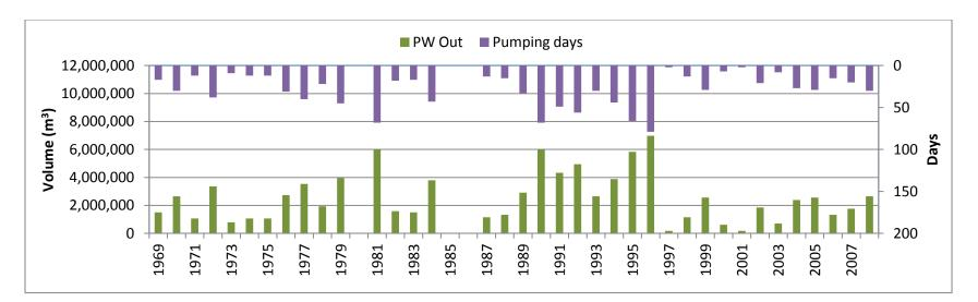
Figure 51: Water Quantity Pumped out from the Marsh and Pumping Days under Hemi Marsh Scenario
