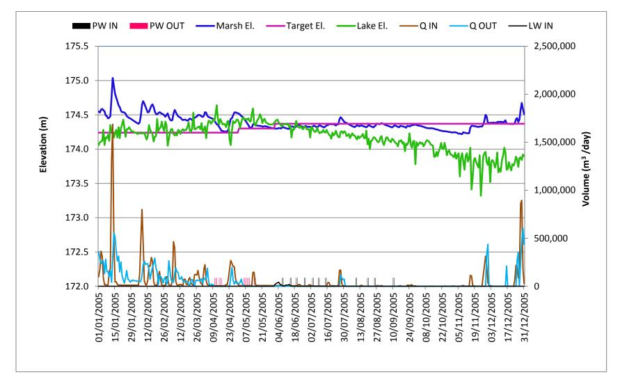
Figure 19: Daily Water Levels, flows and Pumping Water Plot for Hemi Marsh in a dry Year, 2005 Condition
