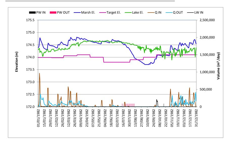
Figure 3: Daily Water Levels, flows and Pumping Water Plot for Open Water Marsh in a Dry Year, 1982 Condition
