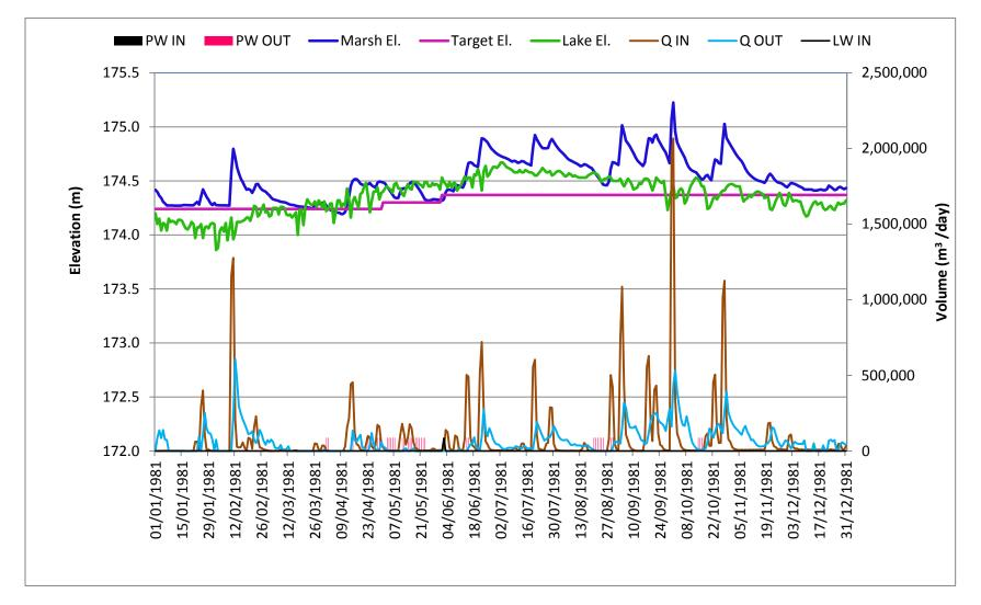
Figure 26: Daily Water Levels, flows and Pumping Water Plot for Hemi Marsh in a Wet Year, 1981 Condition
