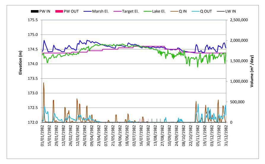
Figure 30: Daily Water Levels, flows and Pumping Water Plot for Overgrown Marsh in a Dry Year, 1982 Condition
