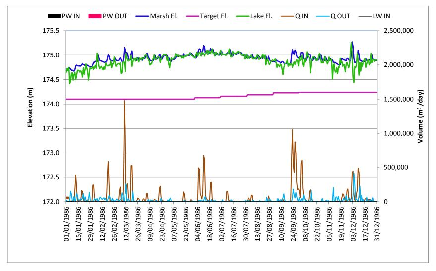
Figure 16: Daily Water Levels, flows and Pumping Water Plot for Open Water 2 Marsh in a Wet Year, 1986 Condition
