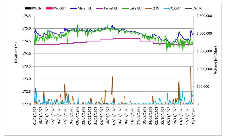
Figure 33: Daily Water Levels, flows and Pumping Water Plot for Overgrown Marsh in an Average Year, 1973 Condition
