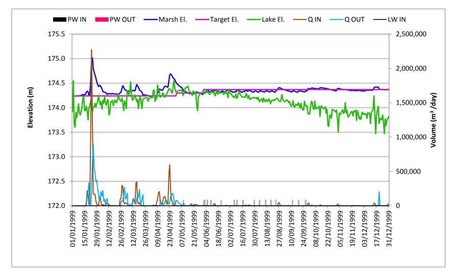
Figure 20: Daily Water Levels, flows and Pumping Water Plot for Hemi Marsh in a dry Year, 1999 Condition
