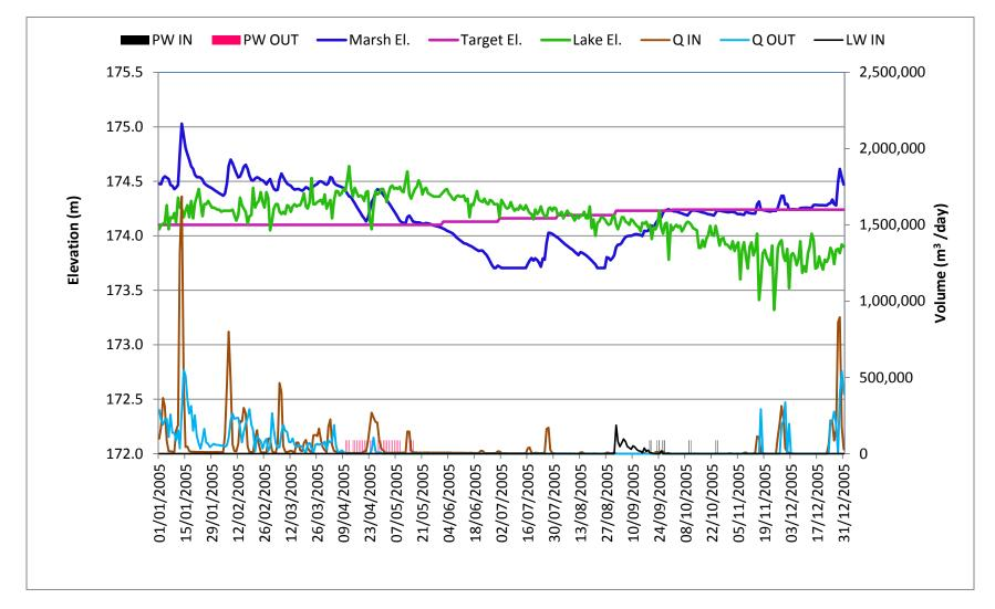
Figure 10: Daily Water Levels, flows and Pumping Water Plot for Open Water 2 Marsh in a Dry Year, 2005 Condition
