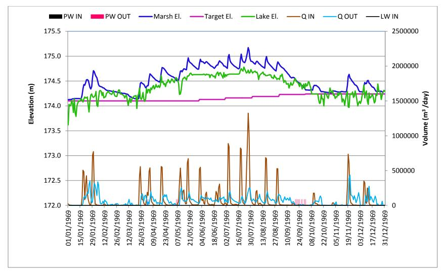
Figure 18: Daily Water Levels, flows and Pumping Water Plot for Open Water 2 Marsh in a Wet Year, 1969 Condition
