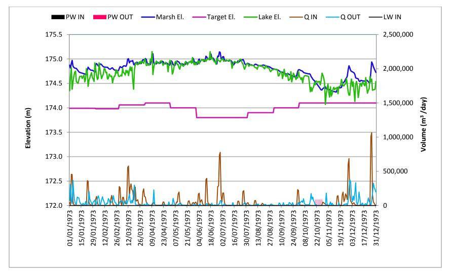
Figure 6: Daily Water Levels, flows and Pumping Water Plot for Open Water Marsh in an Average Year, 1973 Condition
