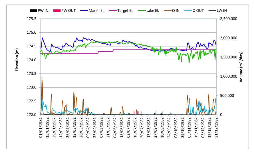
Figure 21: Daily Water Levels, flows and Pumping Water Plot for Hemi Marsh in a dry Year, 1982 Condition
