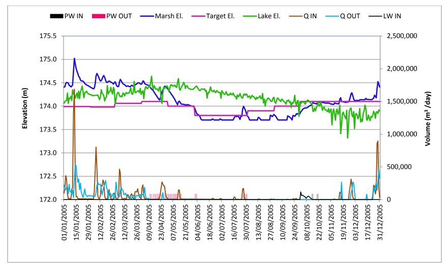
Figure 1: Daily Water Levels, flows and Pumping Water Plot for Open Water Marsh in a Dry Year, 2005 Condition
