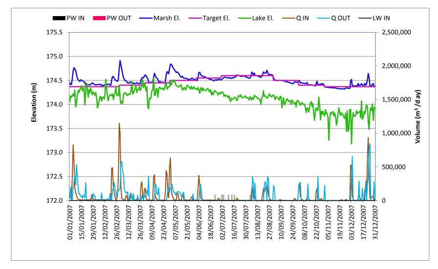
Figure 31: Daily Water Levels, flows and Pumping Water Plot for Overgrown Marsh in an Average Year, 2007 Condition
