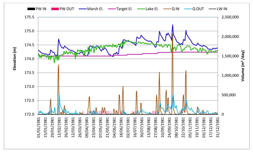
Figure 17: Daily Water Levels, flows and Pumping Water Plot for Open Water 2 Marsh in a Wet Year, 1981 Condition
