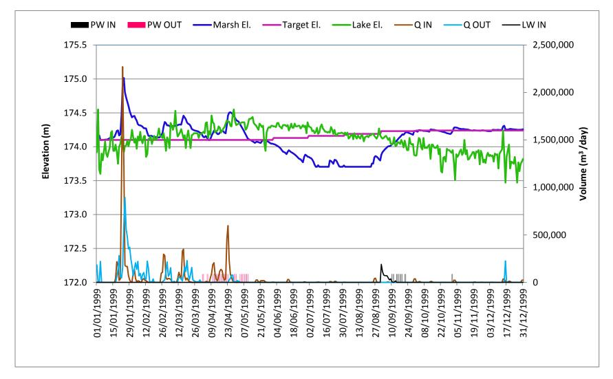
Figure 11: Daily Water Levels, flows and Pumping Water Plot for Open Water 2 Marsh in a Dry Year, 1999 Condition
